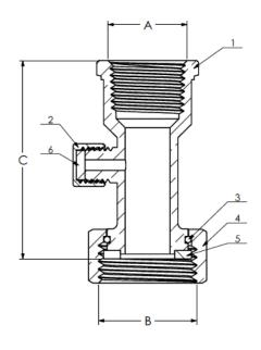
Specifications: Designed for residential, commercial or industrial use with water, oil or gas. Threaded ends comply with ANSI B1.20.1
