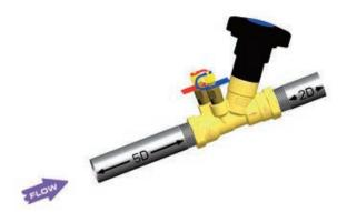
Care should be taken when installing Fig. S1810 (solder end valve) to ensure that the flame is directed away from the center of the valve (valve seat and seals) and also from the P/T ports (seals). This will reduce the risk of damaging the valve seals due to over heating.
