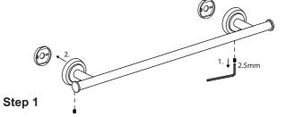
Loosen the set screw on the accessory and remove the backing plates. Position the accessory against the wall and mark outline with pencil.
