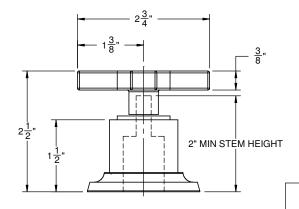
THRU HOLE SPECIFICATIONS RECOMMENDED MIN MAX VALVE: Ø1-1/8" Ø1-3/8" Ø1-5/8" DIVERTER: Ø1-1/2" Ø1-1/2" Ø1-5/8"
